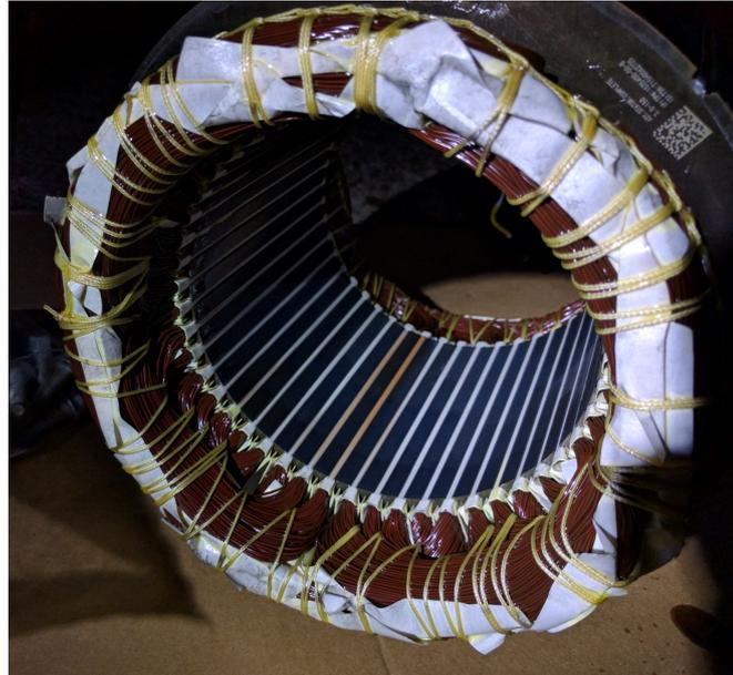
Fig. 1.12: Tesla Model S stator steel pack with winding. Reprinted from [16].
