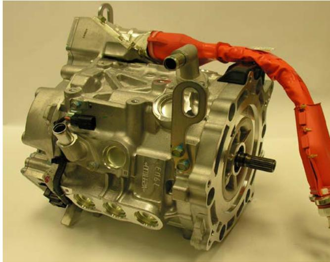
Fig. 1.6: Nissan LEAF complete motor body. Reprinted from [13].
