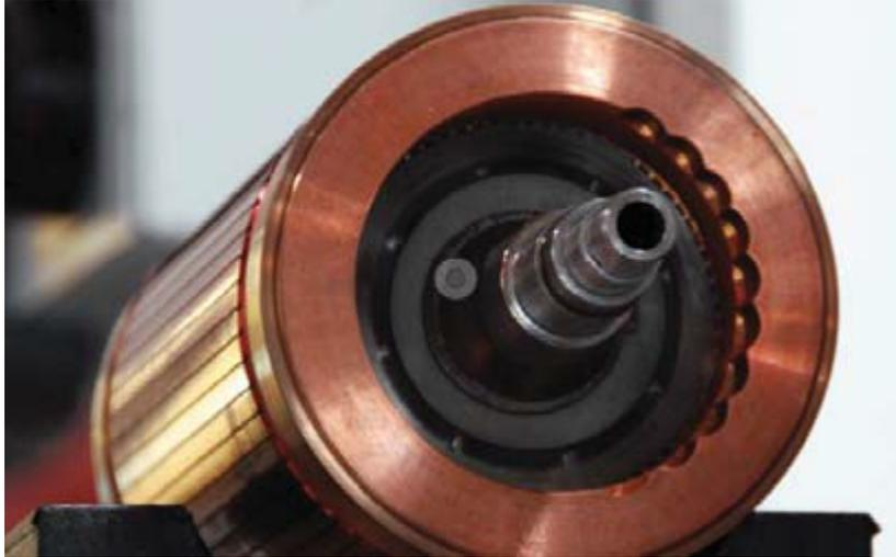
Fig. 1.11: Tesla Model S rotor. Reprinted from [16].
