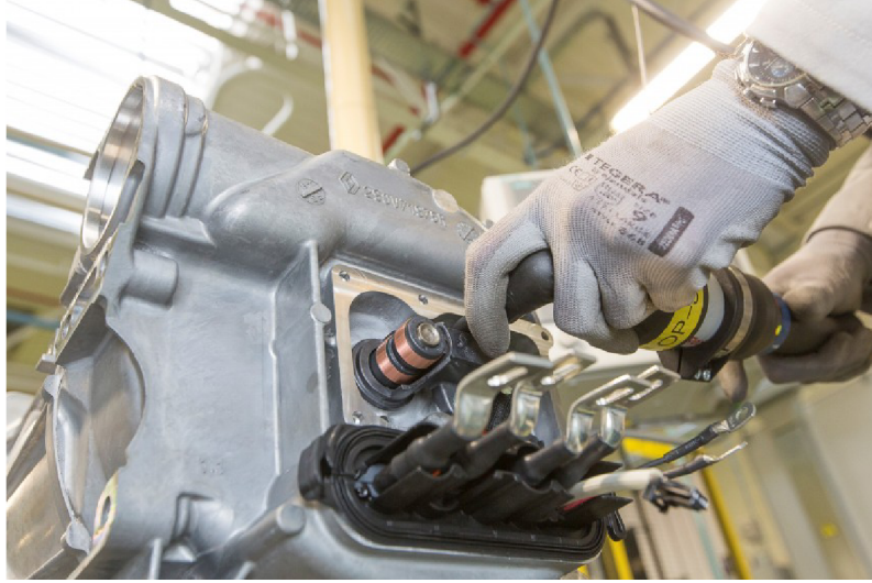
Fig. 1.17: Renault R240 rotor slip rings detail. Reprinted from [21].
