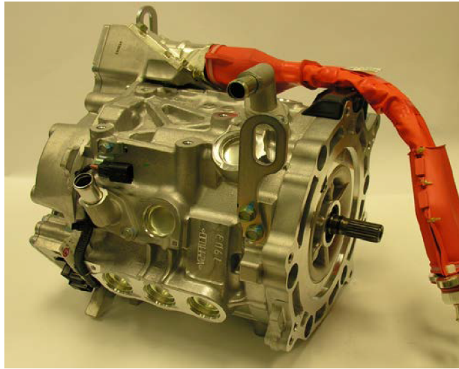
Fig. 1.6: Nissan LEAF complete motor body. Reprinted from [13].
