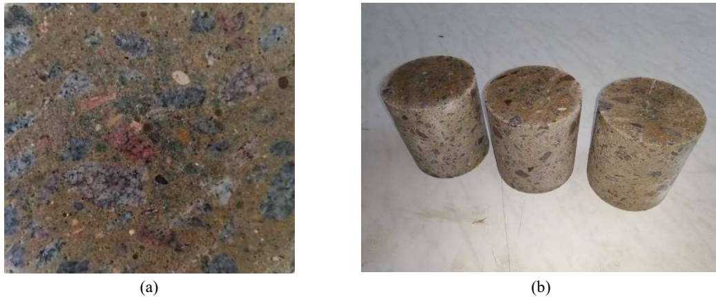
Figure 26: Example of AAC's structure (a) and core-drill samples (b).
