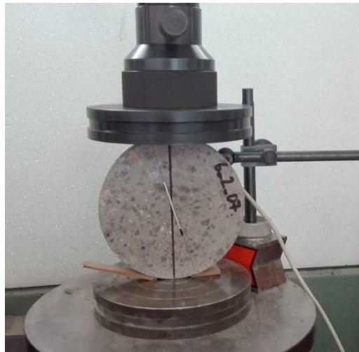
Figure 29: Experimental set-up of BDCN specimen ( a/R = 0.4 \alpha = 20^\circ ).
