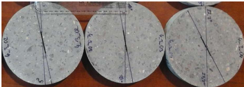
Figure 32: BDCN specimens with marked notch inclination angles with relative notch lengths a/R of 0.267.
