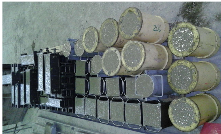
Figure 23: Fresh C 50/60 mixture poured into moulds.
