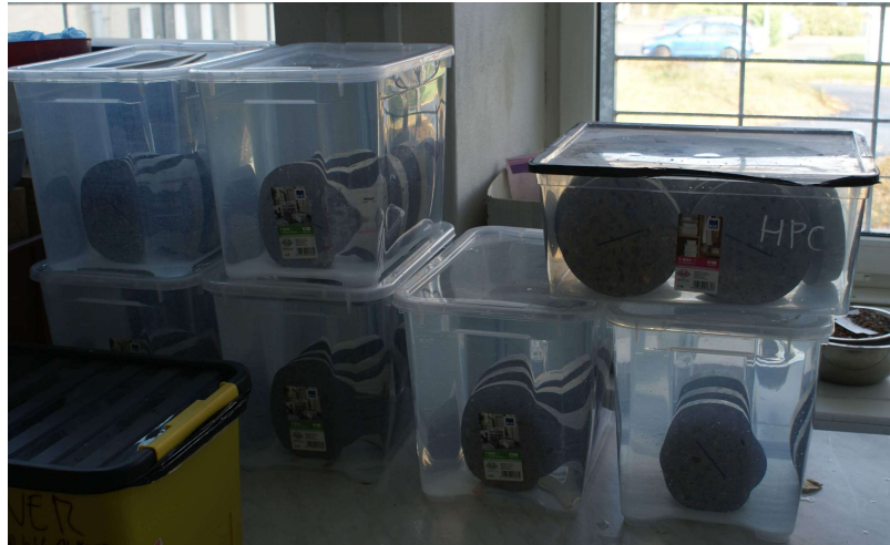
Figure 39: Prepared BD and BDCN specimens stored in plastic containers filled with water and chloride solution in a laboratory room with constant room temperature.
