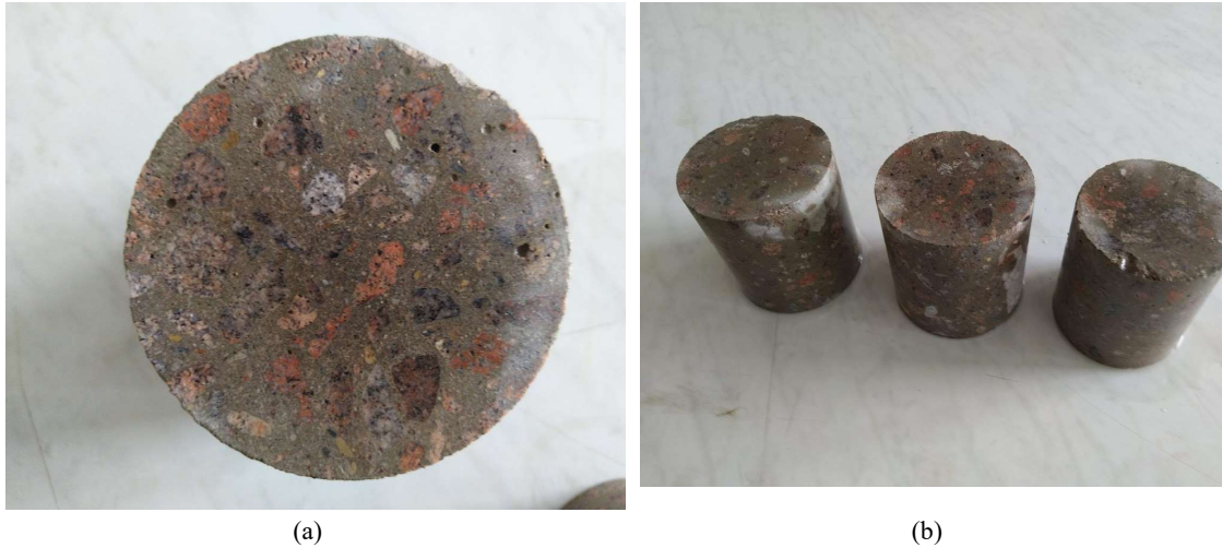
Figure 25: Example of HPC's structure (a) and core-drill samples (b).
