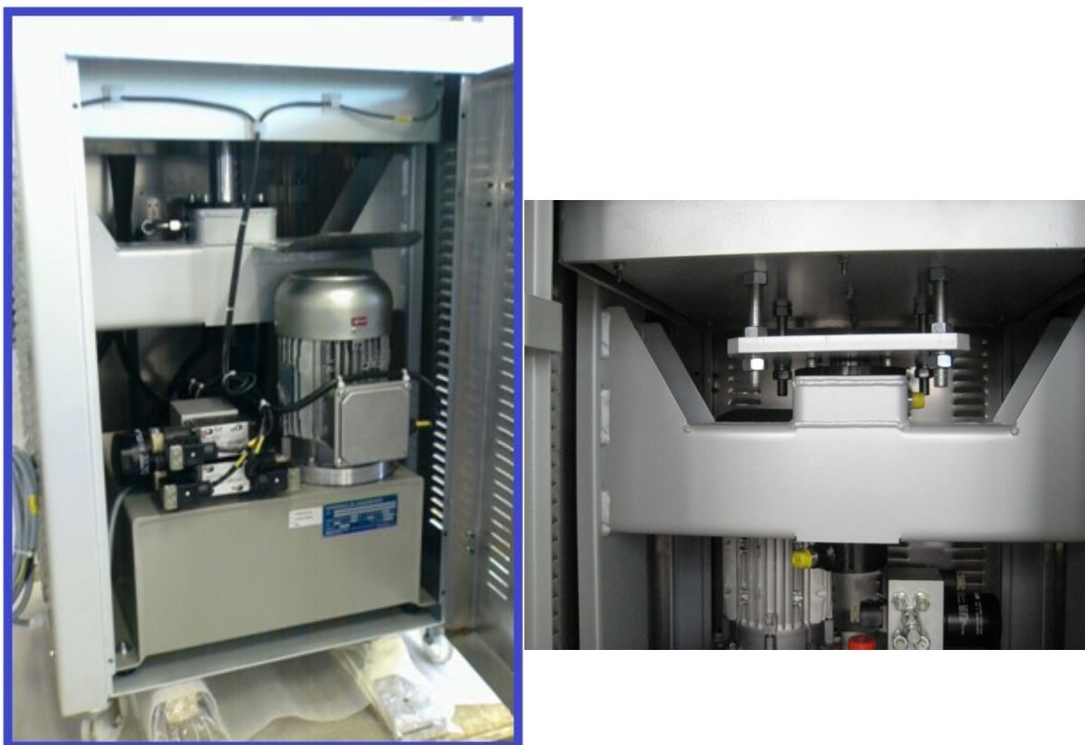
Obr. 2 Detail hydrauliky lisu stroje RONDOPRESS.
