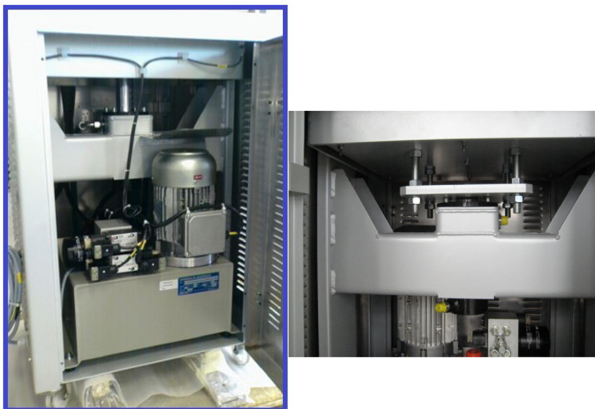
Obr. 2 Detail hydrauliky lisu stroje RONDOPRESS.
