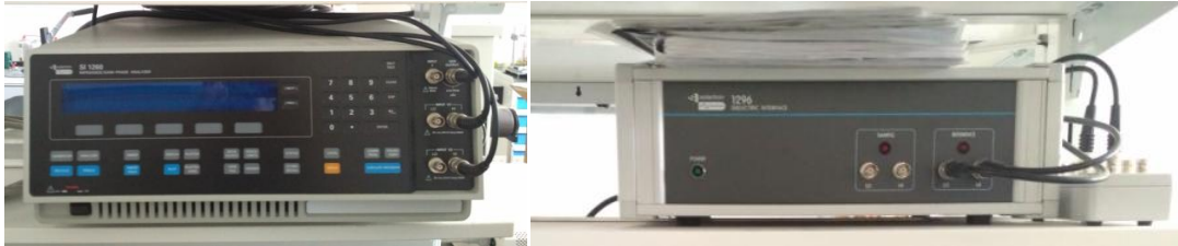
Obr. 25: 1260A Impedance/Gain-Phase Analyzer (vlevo) a 1296A Dielectric Interface System Solatron Analytical (vpravo)
