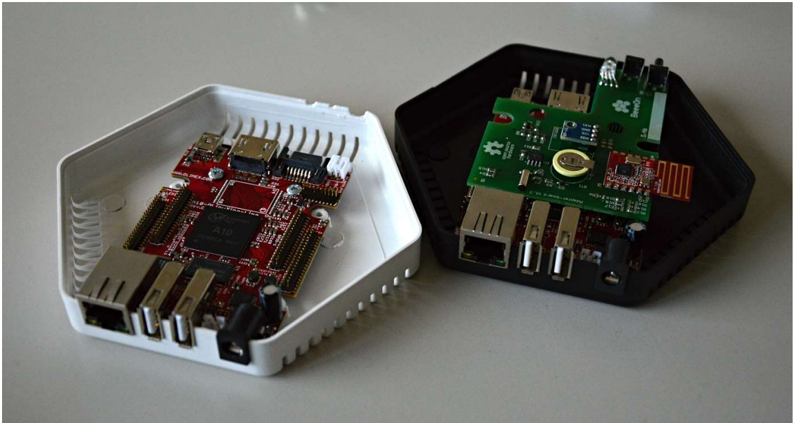
Figure 2.2: Photo of Olimex board A10 on which the BeeeOn system runs [18]
