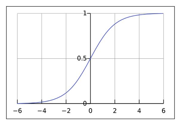
The sigmoid function generates some sort of outputs in the positive numbers realm ranging from 0 to 1. We can comprehend it as squashing  $(-\infty, +\infty)$  to (0,1) — large size negative numbers turn ~0, and large size positive numbers turn ~1.
