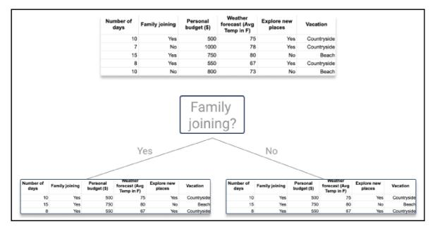
A simple illustration of a decision tree with lets say with tree nodes, the first node being root node and the reaming two leaf nodes.
