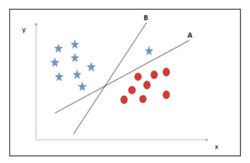
In this case the hyper-plane B has what is called classification error and hyper-plane A has been classified properly. Hence the correct hyper-plane is A.
