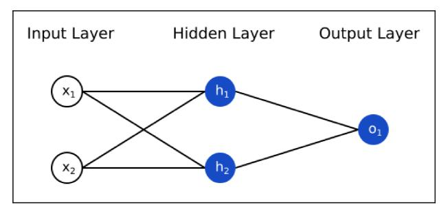
This above mentioned network has two available inputs one called as a hidden layer that has two neurons one of them is h1 and the other h2, and an output layer with 1 neuron (o1). Notice that the inputs for o1 are the outputs from h1 and h2 — that's what makes this a network.
