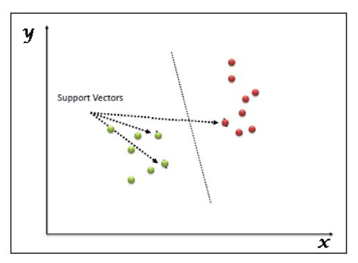
Support Vectors machines just simply represent the orientation of each observation. The Support Vector Machine classifier is a partition that best separates the two classes (hyper-plane or line).
