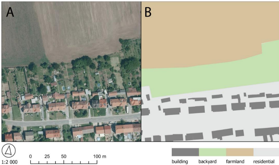
Figure 2 An example of the identification process where an orthophoto input (A) is classified into individual land use types (B)
