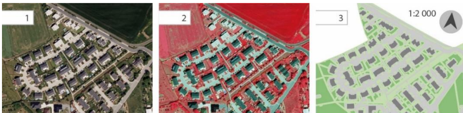
Figure 3 Orthophoto map (1) supplemented with NIR data (2) and the resulting classified layer (3); light green – lawns; dark green – soil surfaces suitable for taller vegetation; grey – paved surfaces; dark grey – built-up areas)
