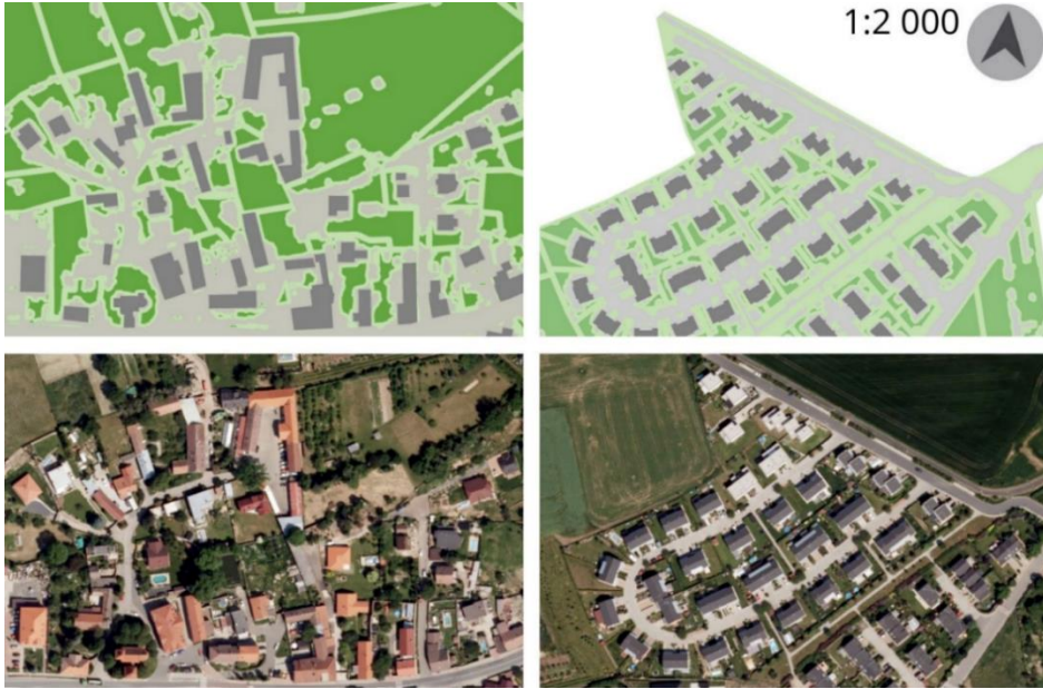
Figure 9 Illustration of the permeability in the historical core built before 1845 (left) and in novel developments built at the beginning of the 21st century (right). Upper images represent the classified layer, the bottom images the orthophoto map. Legend for the classified layer: light green – lawns; dark green – soil surfaces suitable for taller vegetation; grey – paved surfaces; dark grey – built-up areas)
