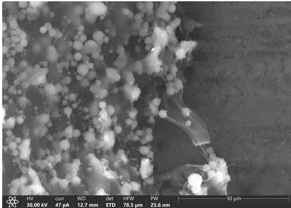
Figure 3.1: Result of electrospinning solution with concentration c = 5\% under a SEM
