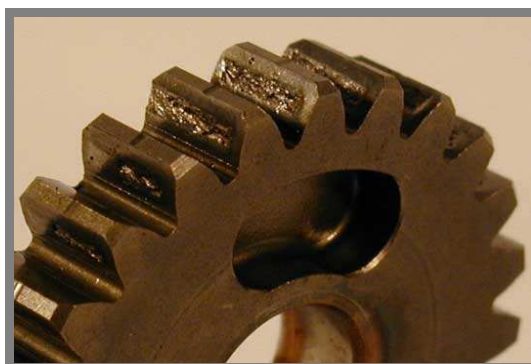
Obr. 4-3 Důlková koroze (pitting) [12]
