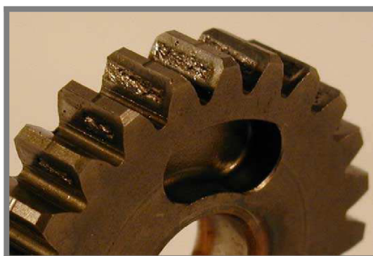
Obr. 4-3 Důlková koroze (pitting) [12]
