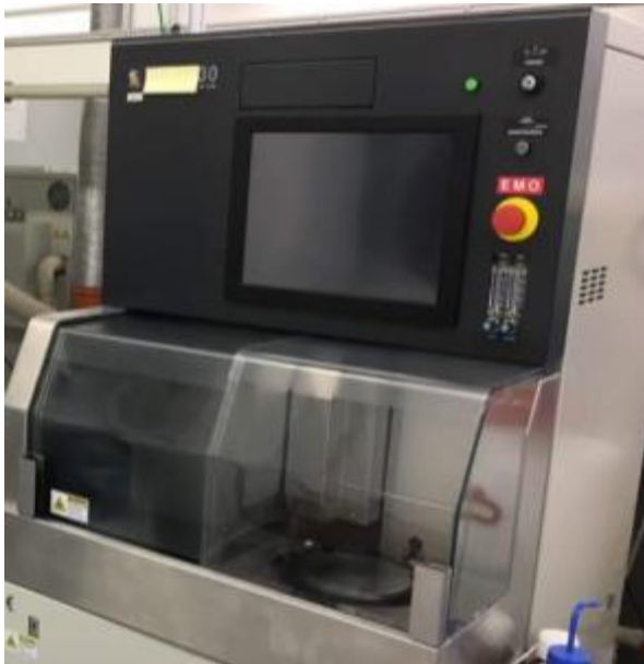
Obr. 23 Diamantová pila pro dicing
