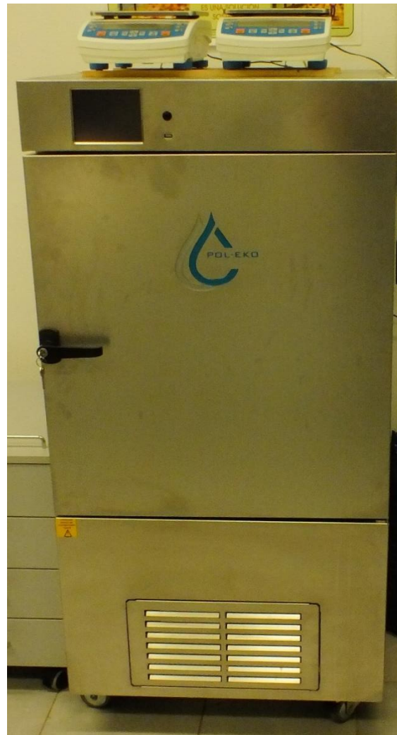
Fig. 12 Climate Box KKP 115 with precision balances
