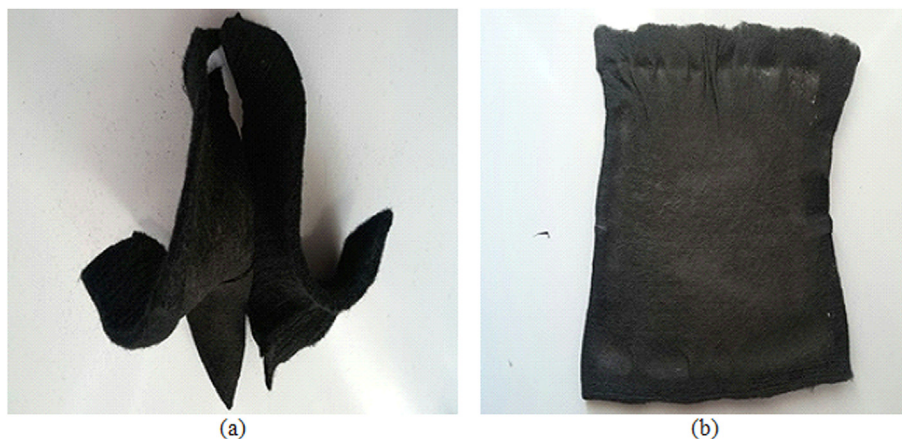
Fig. 3. Activated carbon from stabilization (a) without any pre-tension, (b) with applied pre-tension. (A colour version of this figure can be viewed online.)
