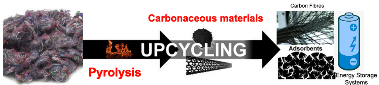
Fig. 1. Upcycling of Fibrous wastes to Carbon-based functional materials. Recreated from [9].
