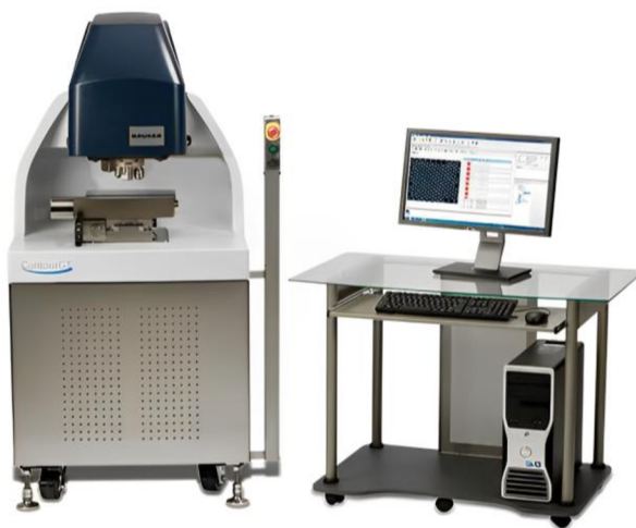
Obr. 4–3 Profilometr Bruker ControuGT-X [45]
