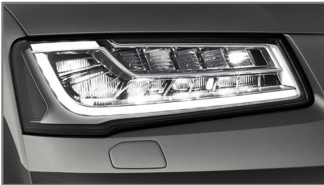
Obr. 2-10 Svetlomet Audi S8 s technológiou Matrix LED [16]
