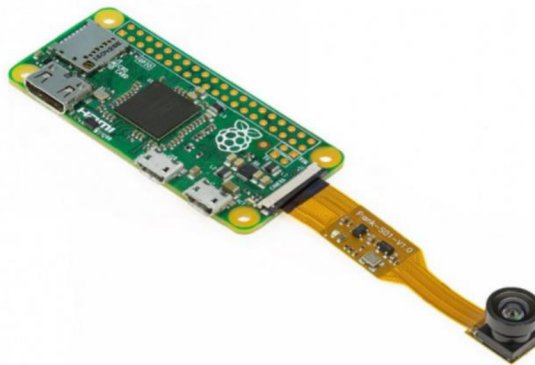
Obr. 3-7 Raspberry Pi Zero a 5Mpx kamera s 160° uhl'om záberu [2]
