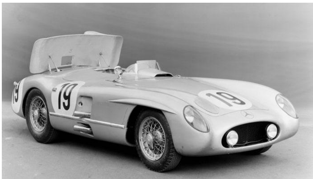
Obr. 3.14 Mercedes-Benz 300 SLR s vysunutou aerodynamickou brzdou [34]
