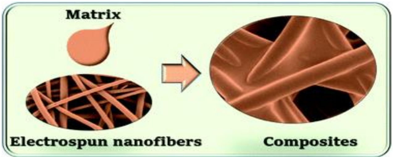
Figure 6: Schematic production procedure of composite with electrospun nanofibers [19]
