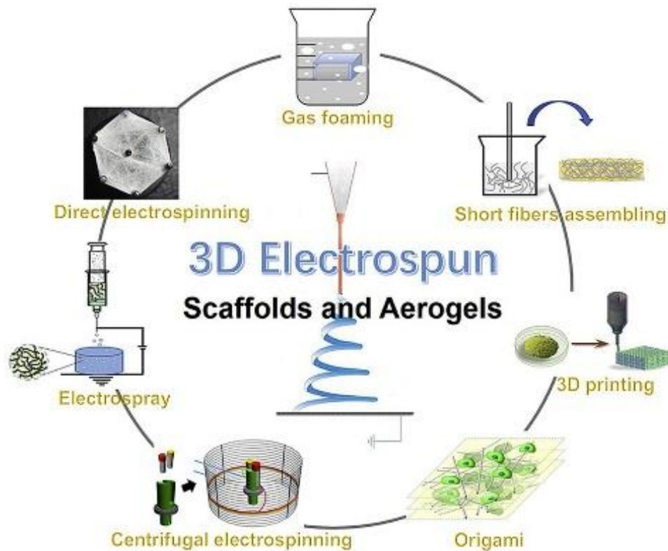
Figure 8: The schematic flow of scaffolds production with electrospun nanofibers [22]
