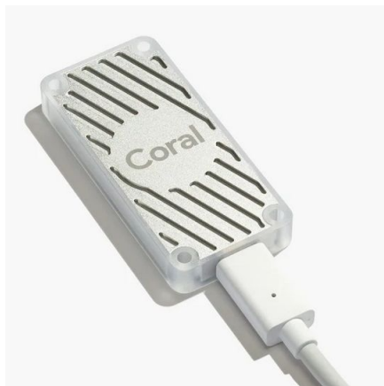
Obr. 4.3: Google Coral - USB Accelerator [5]
