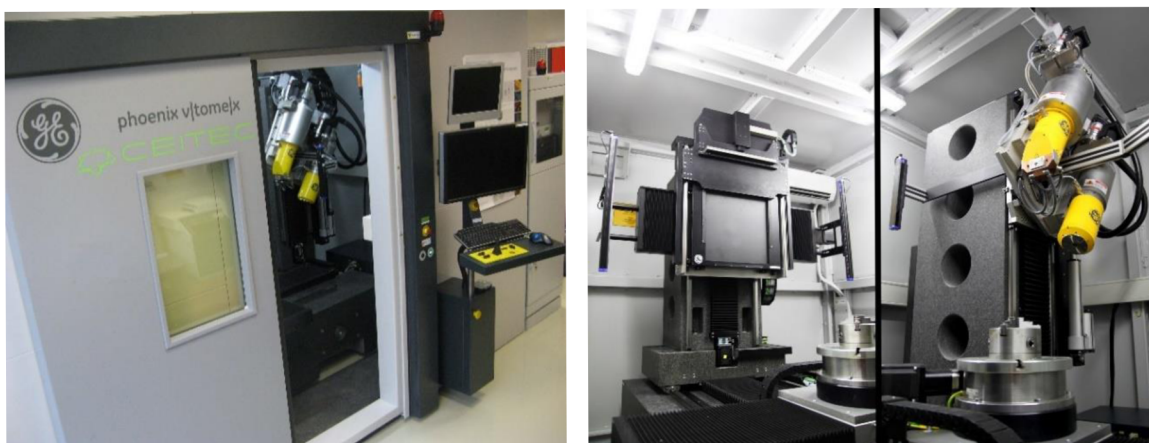
Obr. 41) GE phoenix v|tome|x L240 [2]
