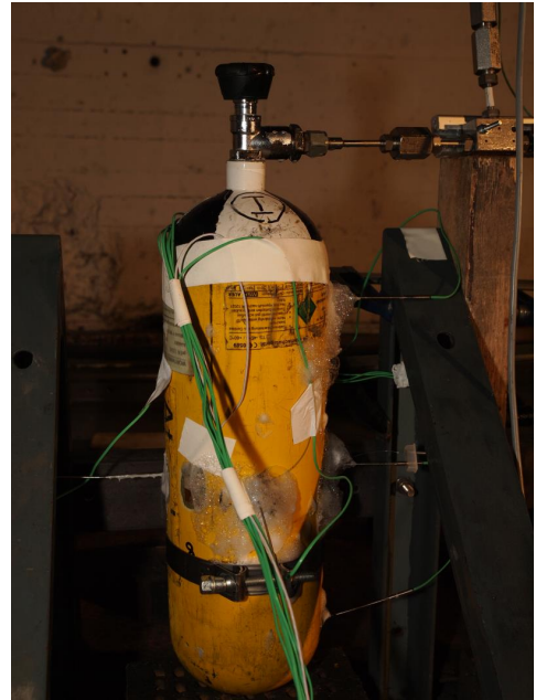
Figure 2 - drilled bottle with sensors
