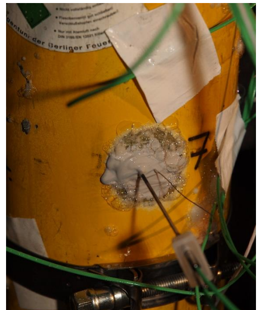
Figure 17 – showing drilling of sensors in the flask
