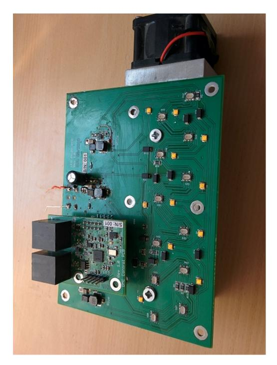
Figure 10.7: Both PCBs connected together
