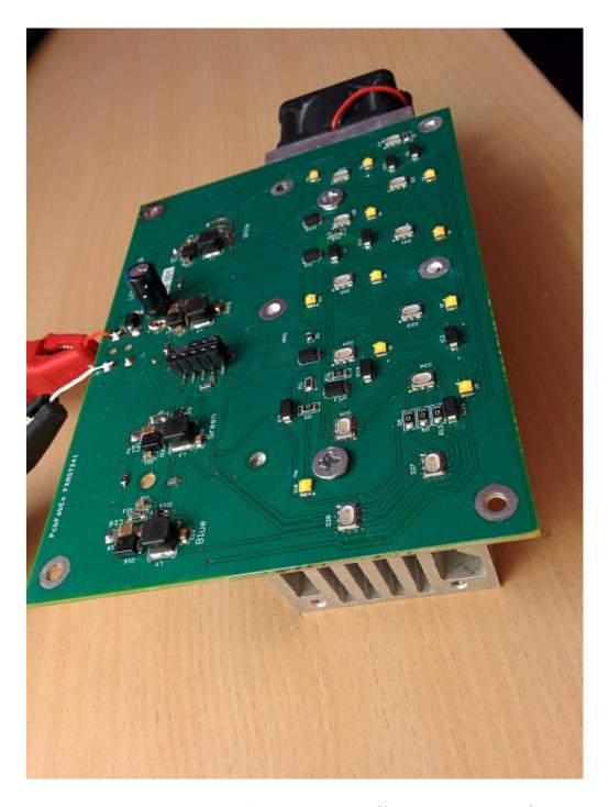
Figure 10.5: The Power Board (for testing purposes)
