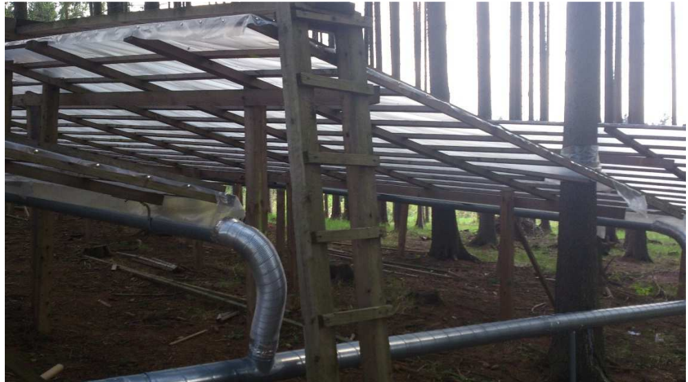
Photo 1 – Experimental plot covered by roof system. There can be seen gutter, through with rainfall was taken out from the plot. Ladder was used to climb on the roof and empty and change window traps. (Mladenović Strahinja, 2013)
