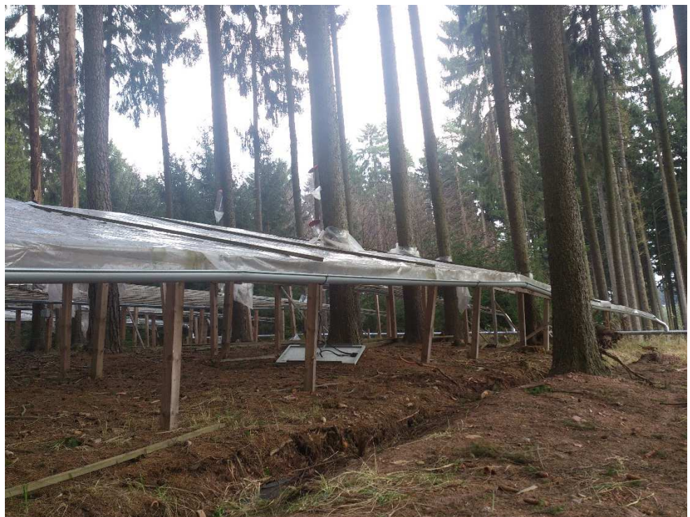
Photo 2 – Experimental plot covered by roof system. (Mladenović Strahinja, 2013)
