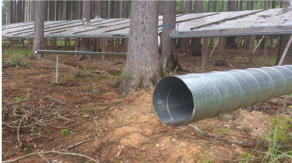
Photo 7 – Complex of gutters was taking water input far away from experimental plot. (Mladenović Strahinja, 2013)
