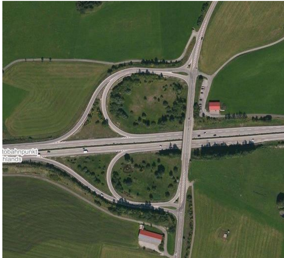
Appendix 12 An example of half-clover intersection. Source: [34]
