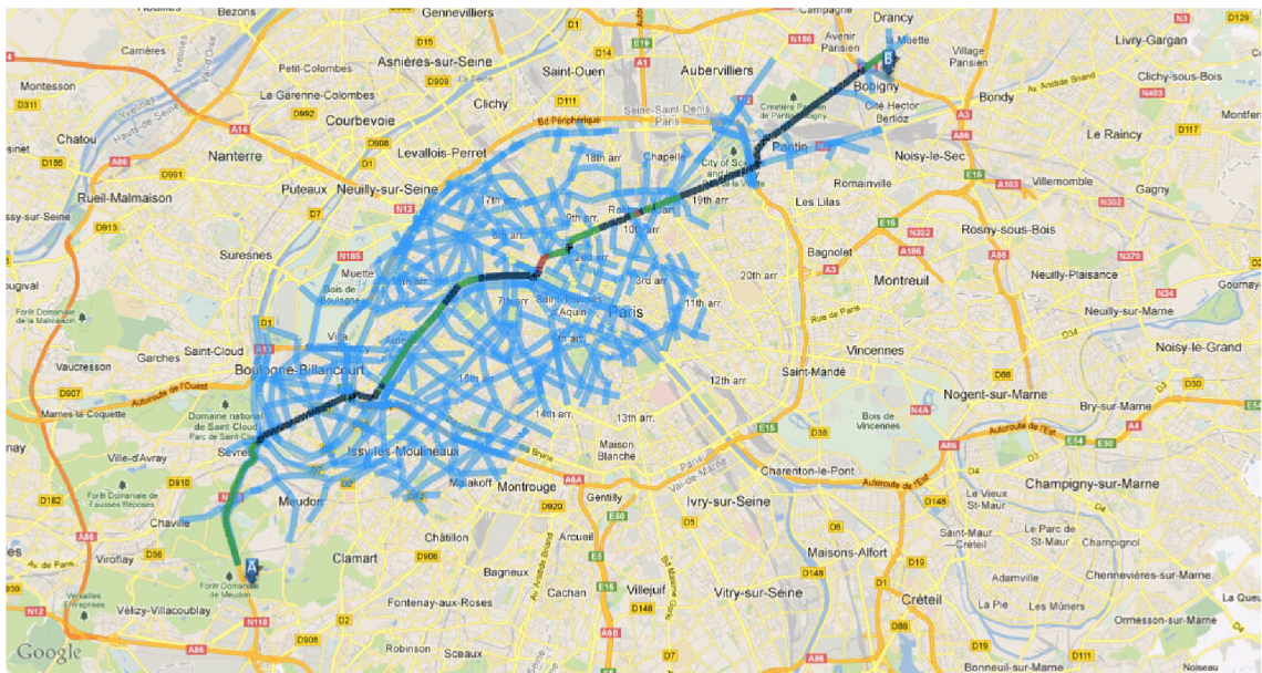
Fig. 4.2: Schematic representation of the search space of the A* algorithm
