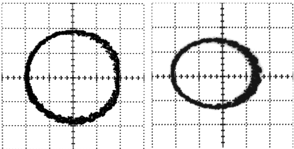
Fig. 3.16. Experimental illustration of amplitude correction and rotational misalignment of the PBS 1.
