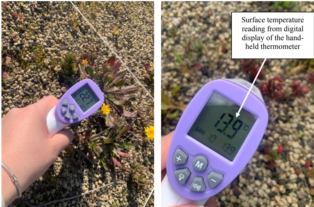
Figure 17. Hand-held digital thermometer (YM-6688) Source: Author
