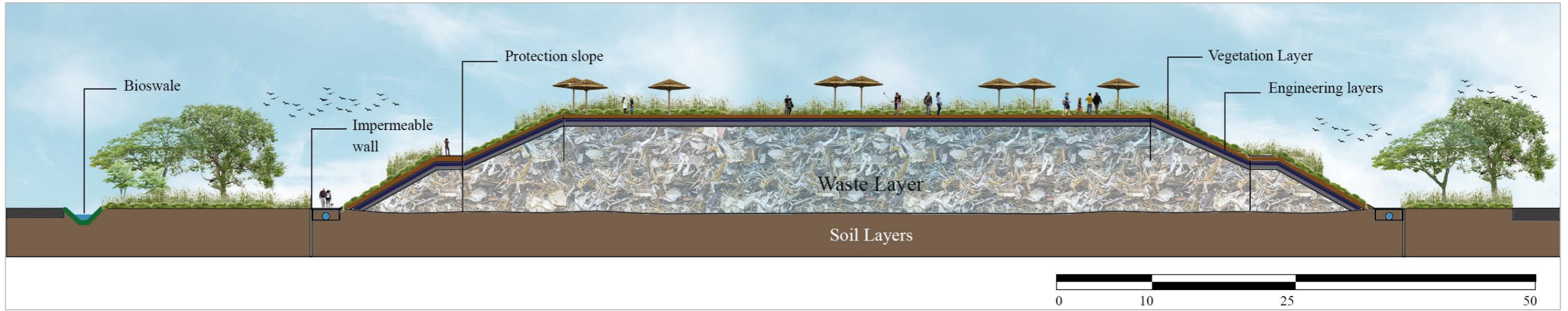
Appendix 2. Compacted waste section
