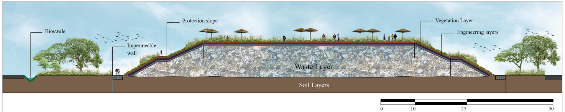
Appendix 2. Compacted waste section
