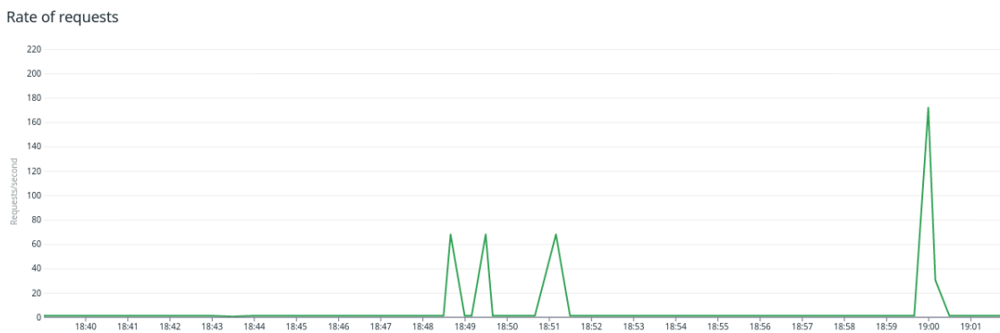
Fig. A.10: Rate of requests during a flood attack with my module turned off.
