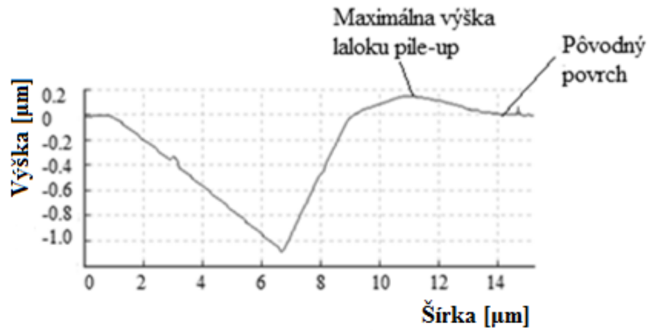
Obr. 36 Profil vtláčku (DP 600); F_{max} = 100 \text{ mN} [70]
