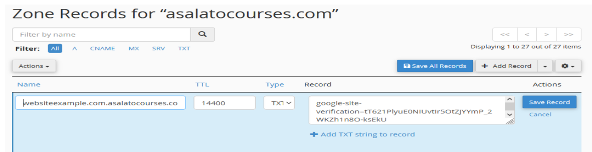
Figure 38 Configuring DNS Settings for Domain Verification using Namecheap's cPanel Zone Editor (own source)
