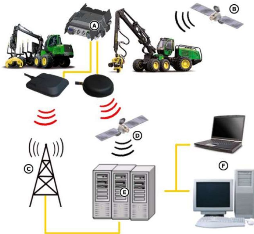
Picture no:1 Illustration of the harvester data communication process. (John Deere 2014)
