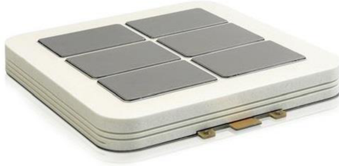
Figure 17: Typical appearance of ABB's IGBT press-pack [39]
