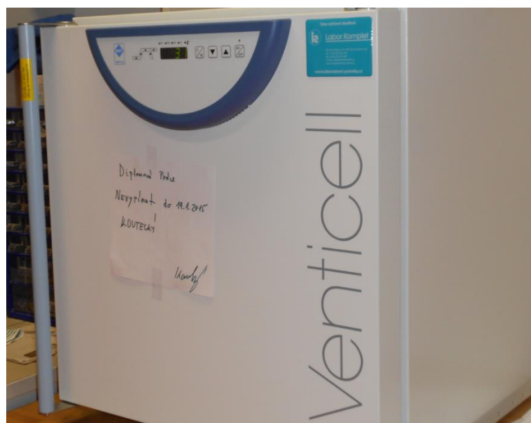
Obr. 5.4 Sušárna Venticell BMT MMM Group.
