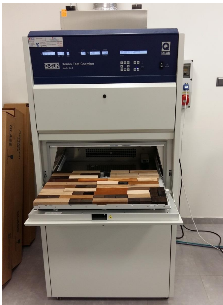
Obr. 9: Xenon Test Chamber, Model Xe – 3, Q – Sun, Q – Lab (Pelzerová, 2017).
