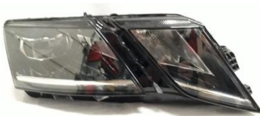
Obr. 21 - Full-LED světlomet (Škoda Octavia III. facelift) [27]
