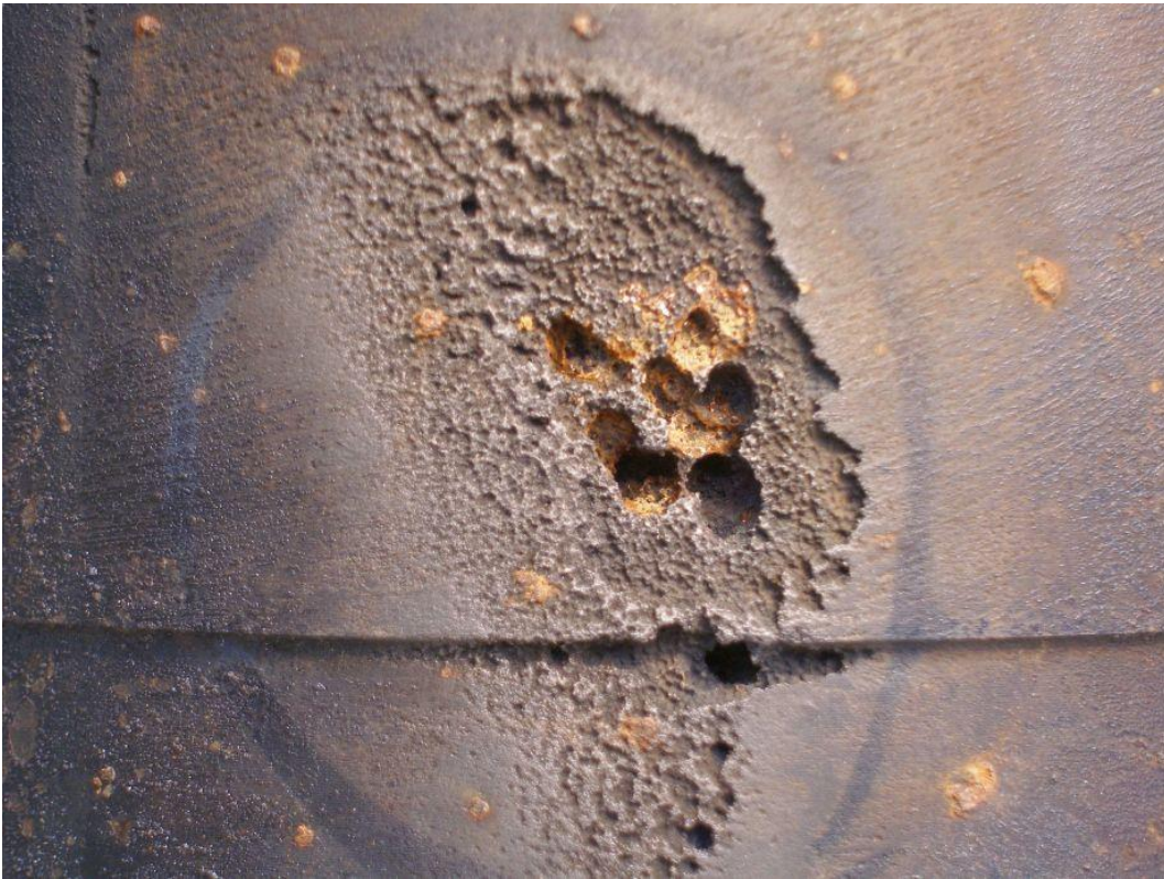
Pitting corrosion – Diesel motor cylinder liner
