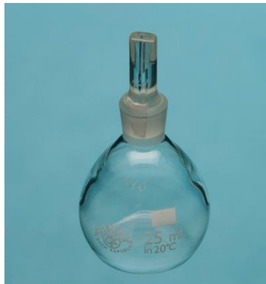
Fig. 5-12 Pycnometer – 25 mL/20 °C 168
