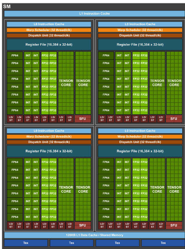
Obr. 2.1: Volta streaming multiprocessor. Prevzaté z: [21].
