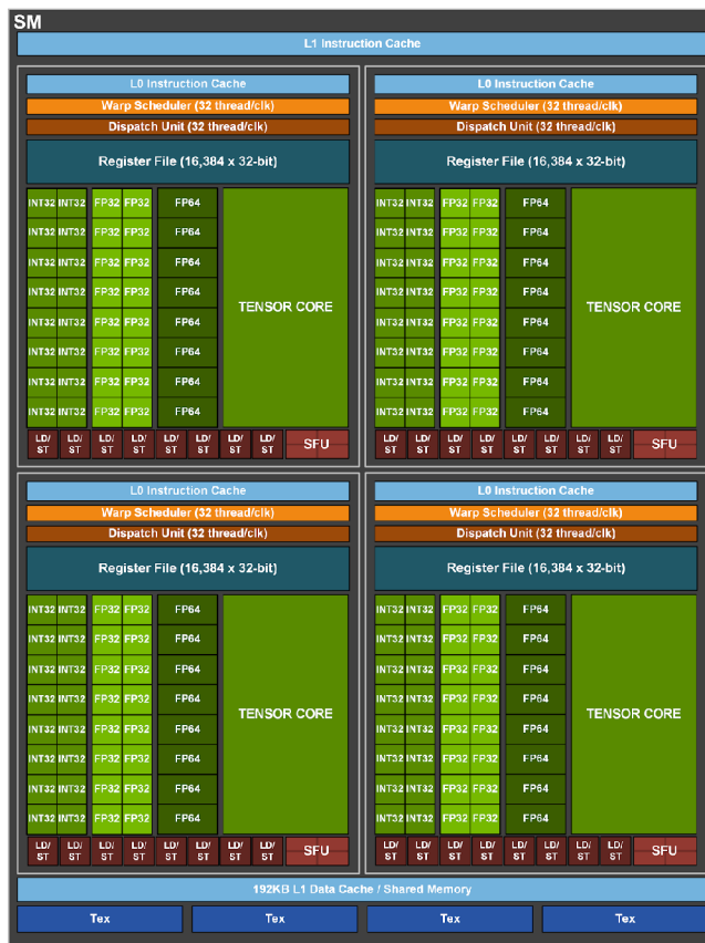
Obr. 2.2: Ampere streaming multiprocessor. Prevzaté z: [9].
