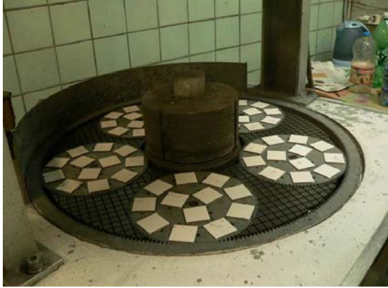
Figure 22 - Ceramic prepared for grinding
