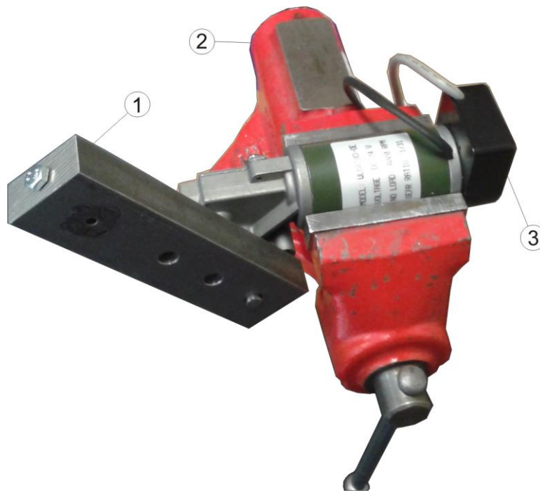
Figure 8, Testing device: 1 - holder, 2 - vise, 3 - DC motor
