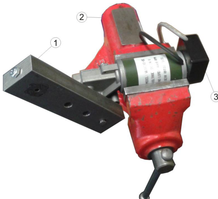
Figure 8, Testing device: 1 - holder, 2 - vise, 3 - DC motor
