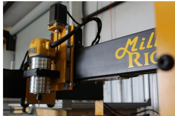
Obr.2.3 Detail osy Y a Z [4].
