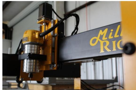
Obr.2.3 Detail osy Y a Z [4].
