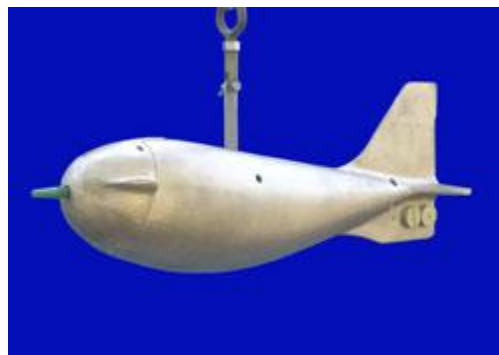
Figure 3. US DH-74 Depth integrating suspended sampler (USGS 2015).
