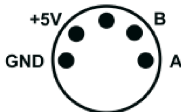
Figure 1.6: 5-pin DIN Encoder pin-out [2]
