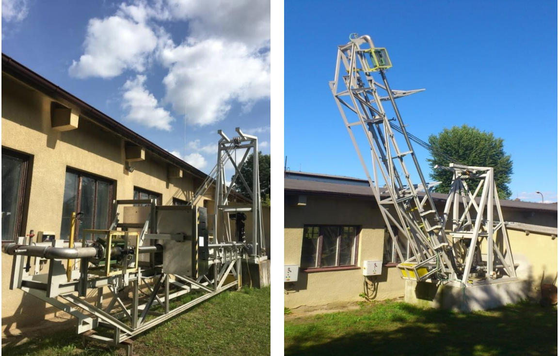
Figures 4–5: The inclinable section of the experimental loop in the horizontal position (left) and inclined position (right).
