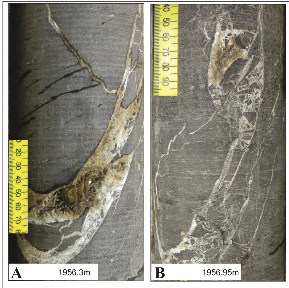
Figure 14 (A and B) Fracture types in cores of limestone and argillaceous limestone from the Shiranish Formation in the Taq Taq oil field (Rashid et al., 2023).
